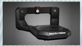
**3D scanners** collect data on the three-dimensional shape and appearance of an object.
