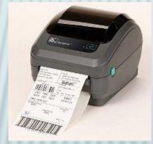
**Thermal printers** work by selectively heating regions of special heat-sensitive paper.
