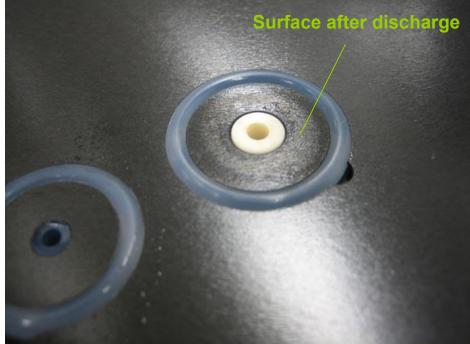
Position of capacitive discharge inside lift up hole
