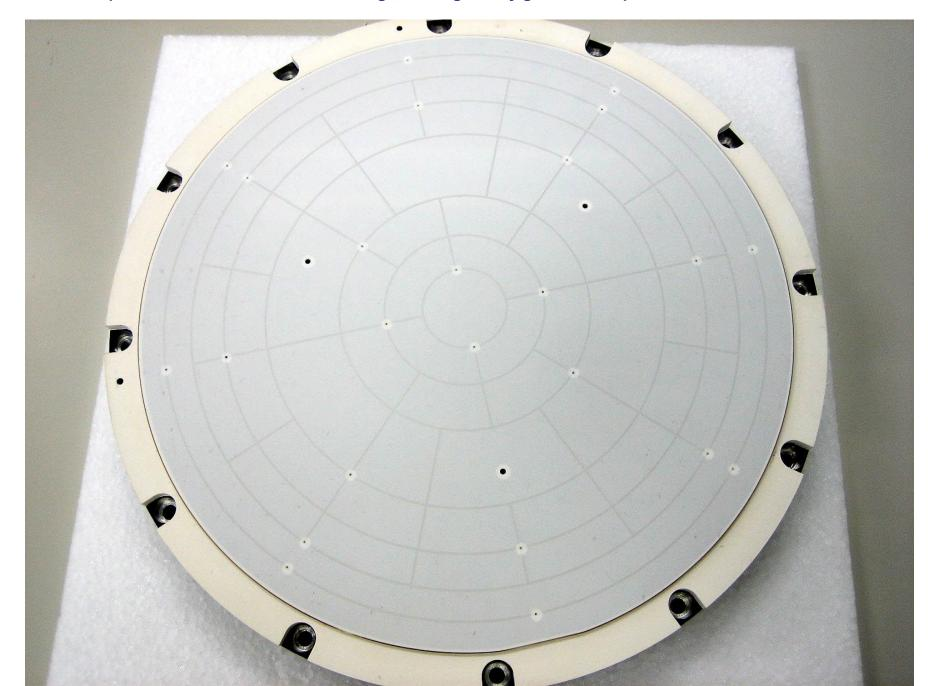
Under cathode parts has no damage too.
