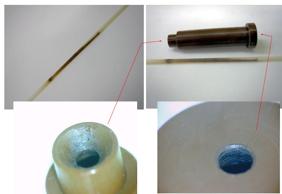
Cathode bottom surface around this lift up hole has traces of RF capacitive discharge too.
