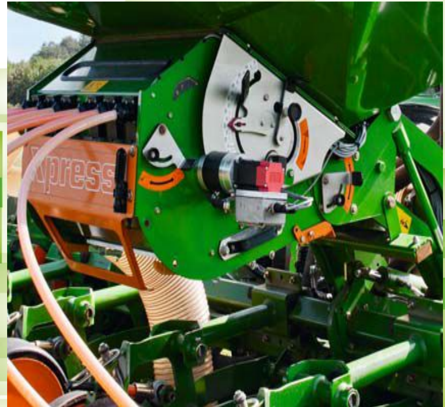
EDX eSeed – detailed view 230 V metering servo-motor
