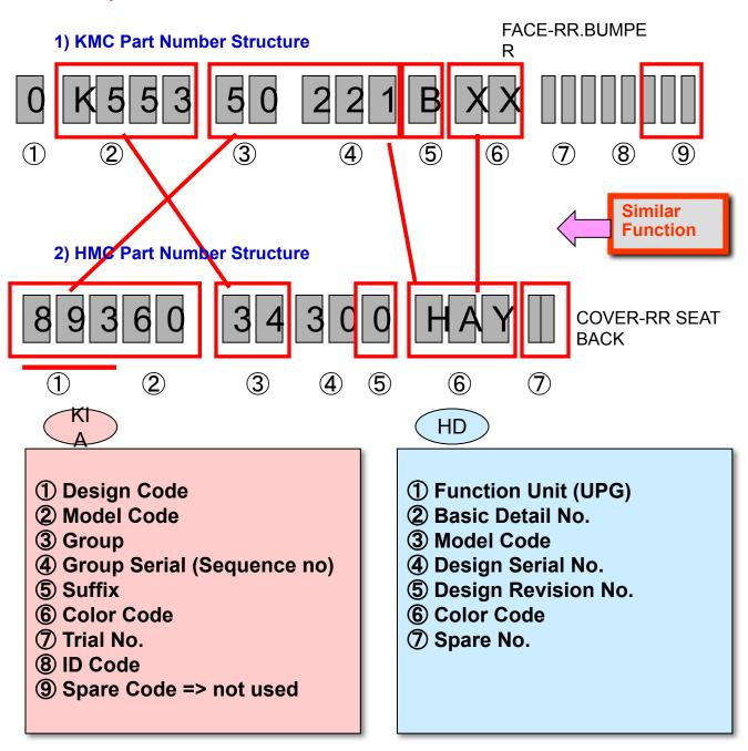
◆ STANDARD PART : KMC => 2<sup>nd</sup> BYTE = '9' ◆ ASSY PART : KMC => 10<sup>th</sup> BYTE = '0' HMC => 1<sup>st</sup> BYTE = '1' or Alphabet
