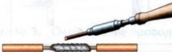
An illustration showing a soldering iron with a blue handle and a metal tip. The tip is applied to the twisted wires, and a grey, wavy substance representing solder is being applied to the joint. |
