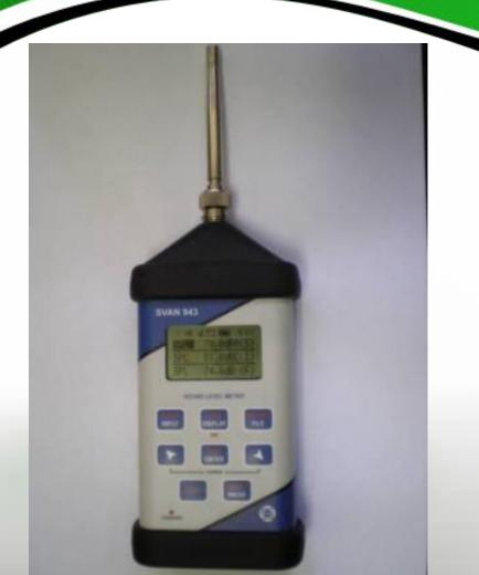
To measure noise using sound level meter: the simplest case, it consists of an amplifier to the input of which is connected a measuring microphone, and to the output of the voltmeter widget in decibels.
