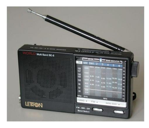
Radio (room radio) receiver device) - a device for reception of electromagnetic waves radio range (that is, with the wave length from a few thousand metres to tenths of a millimeter) followed by conversion to the information of the type for which it could be used.
