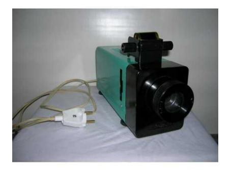
A slide projector is an opto-mechanical device to view photographic slides. Slide projectors became common since the 1950s as a form of entertainment; family members and friends would gather to view slide shows. In-home photographic slides and slide projectors have largely been replaced by low cost paper prints, digital cameras, DVD media, video display monitors, and video projectors.
