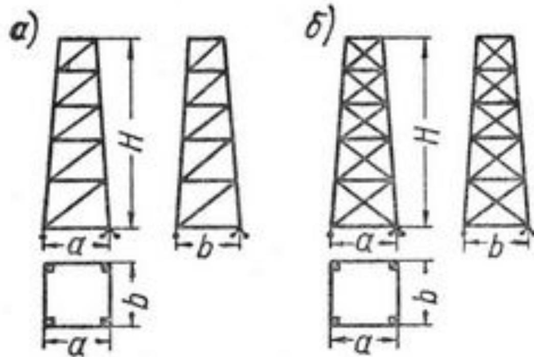
$$\begin{aligned} \text{а} & \text{ — } b/H = 1/1 \div 1/8; H_{\text{макс}} = 40 \text{ м}; \\ \text{б} & \text{ — } b/H = 1/1 \div 1/8; H_{\text{макс}} = 40 \text{ м);} \end{aligned}$$
