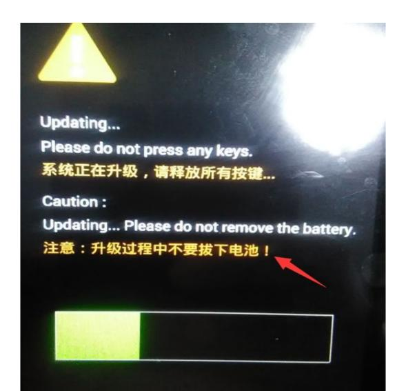
The sixth step: in accordance with the phone prompts the operation, then press the power button to restart the system, there will be boot screen, the whole process of the software upgrade.
