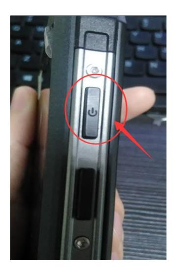
The fourth step: in accordance with the phone prompts, please press the power button to continue, and then press the power button for a long time.
