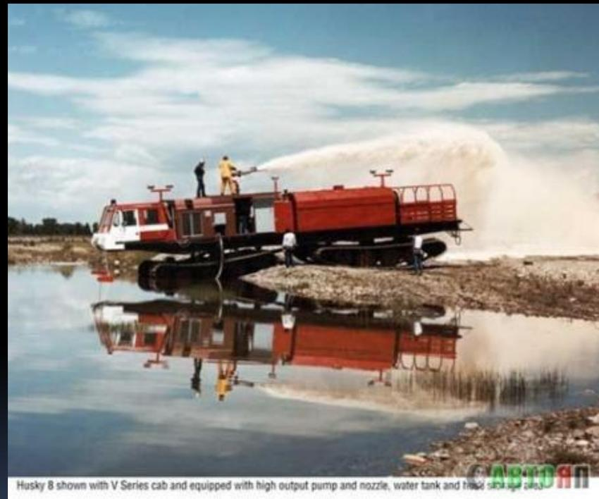
Husky 8 shown with V Series cab and equipped with high output pump and nozzle, water tank and tracks.
