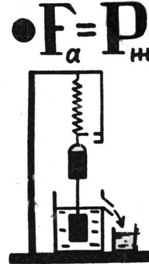
●  $F_a = F_{\text{выт}} = F_2 - F_1 = p_2 S - p_1 S = g \rho_{\text{м}} h_2 S - g \rho_{\text{м}} h_1 S =$
