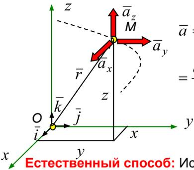
$$\vec{a} = \frac{d^2 \vec{r}(t)}{dt^2} = \frac{d^2}{dt^2} [x(t)\vec{i} + y(t)\vec{j} + z(t)\vec{k}] = \frac{d^2 x}{dt^2} \vec{i} + \frac{d^2 y}{dt^2} \vec{j} + \frac{d^2 z}{dt^2} \vec{k} = a_x \vec{i} + a_y \vec{j} + a_z \vec{k}$$
