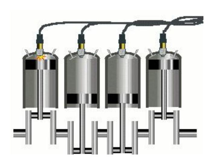
Internal combustion engine - engine in which fuel is burned directly in the chamber (internal) motor. ICE converts thermal energy from the combustion of fuel into mechanical work.
