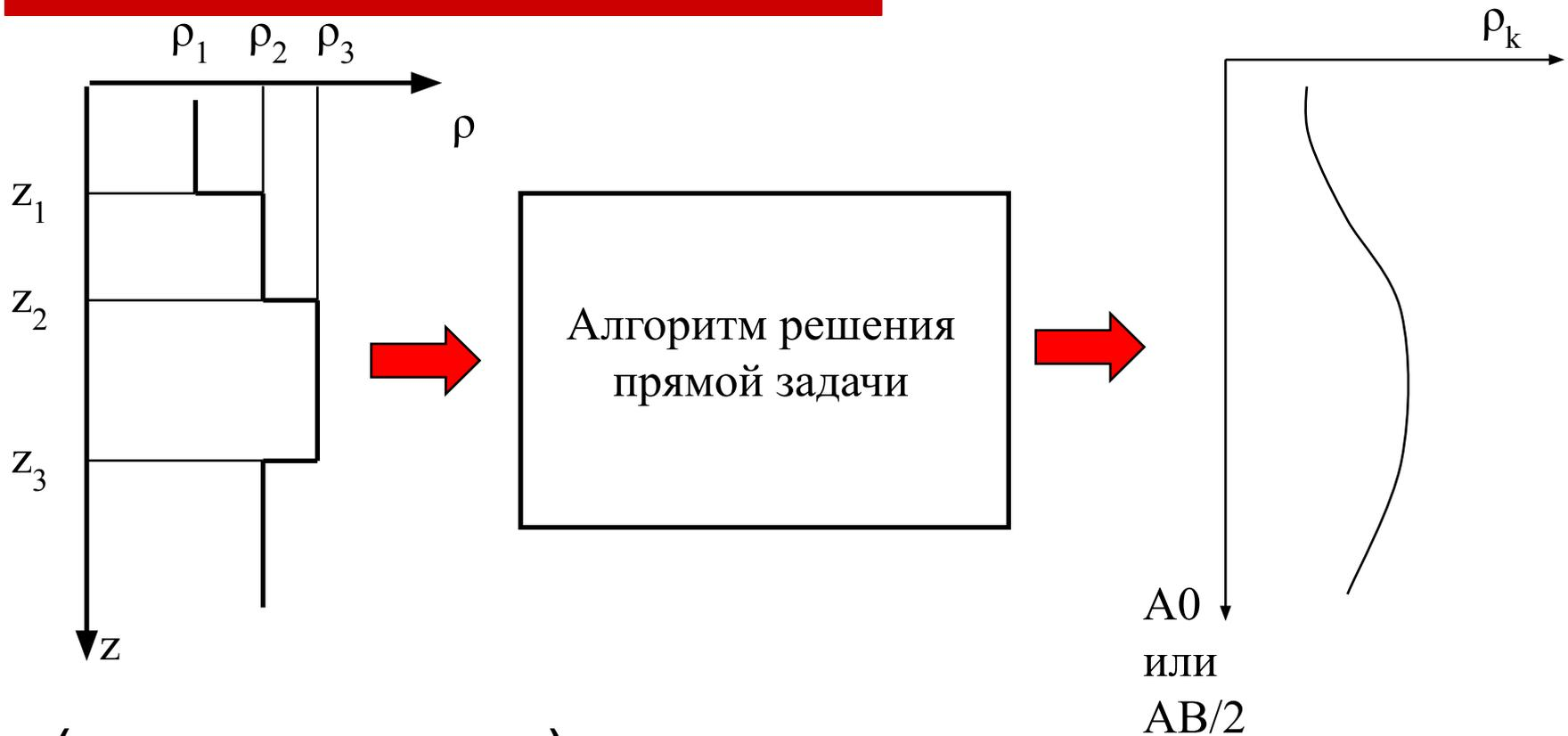
$$\mathbf{p} = (\rho_1 \rho_2 \rho_3 \rho_4 \dots z_1 z_2 z_3 \dots)$$
