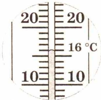
$$\text{цена деления} = \frac{20^{\circ}\text{C} - 10^{\circ}\text{C}}{10} = 1^{\circ}\text{C}$$
