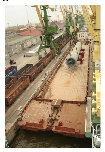
Design works had been carried out and as a result 2 types of barges had been refitted as Roll-on/Roll-off (Ro-Ro) for this very shipment.
