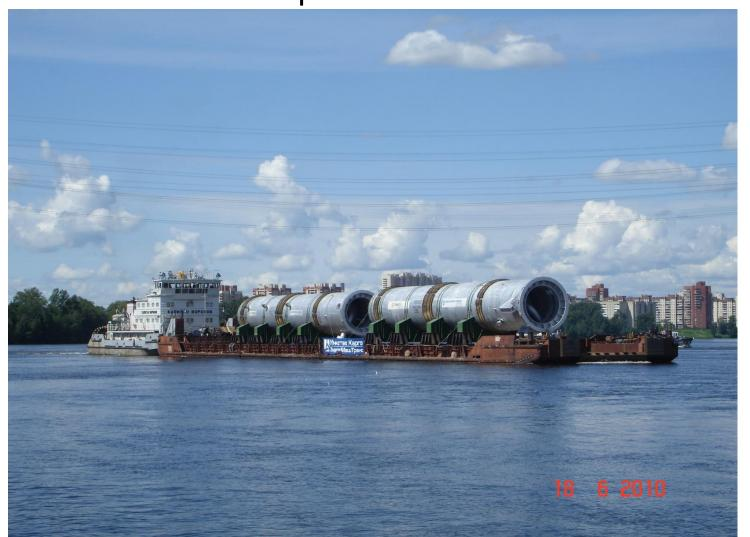
Preparation took about 900 days. New berth on Neva River was built as well as the road leading to it, it had been approved by Russian Railways JSC to close the railway crossing, the barge had been strengthened.
