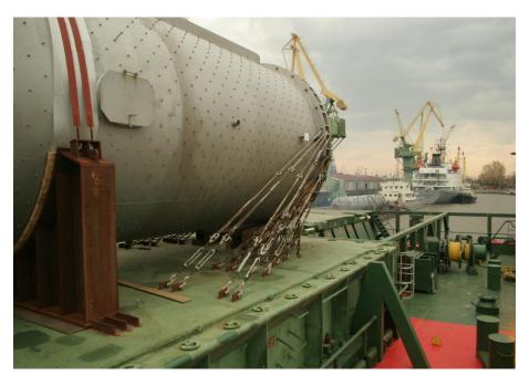
These barges delivered the cargo to berth in Kirishi, which has been specially built for this equipment receipt. All handling operations were carried out by ballasting the barge.
