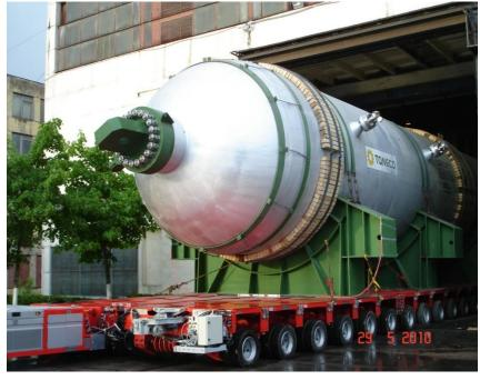
Simultaneous transportation of 2 hydrocracking reactors (**total** weight 2 500 MT - 1250 MT each, 37,5 m. x 7,7 m. x 6,5 m.) for Oil Refining and Petrochemical Complex TANECO in Nizhnekamsk.
