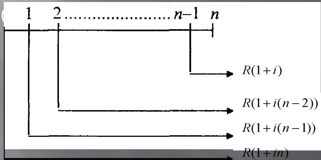
$$\begin{aligned} S &= R \sum_{t=0}^{n-1} (1 + i(n-t)) = R \cdot [1 + n \cdot i] + R \cdot [1 + (n-1) \cdot i] + \dots + R \cdot [1 + i] \\ &= R \left[ n + i \cdot (1 + 2 + \dots + n) \right] = R \left[ n + i \frac{n \cdot (n+1)}{2} \right] \end{aligned}$$
