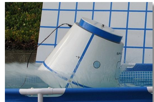
1:3 scale Model Splash Test
