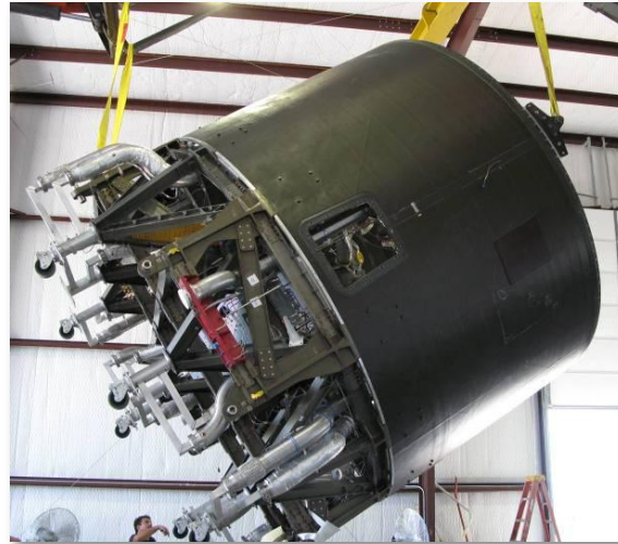
Thrust frame & plumbing for nine engines
