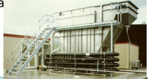
Dissolved air flotanon system for a carring industrial wasterwater.
