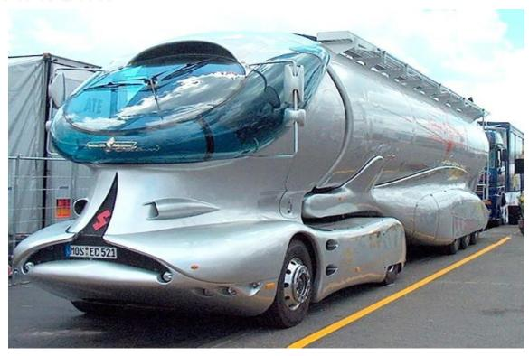
IN THE FUTURISTIC CONCEPT OF THE CAR, DESIGNED TO TRANSPORT GOODS OVER LONG DISTANCES, THERE ARE NO BATTERIES OR HYDROGEN FUEL CELLS. INSTEAD, IVECO EQUIPPED THE Z TRUCK WITH AN ENGINE POWERED BY TRADITIONAL LIQUEFIED NATURAL GAS IN THE FORM OF BIOMETHANE DERIVED FROM PURIFIED BIOGAS, WHICH WILL REDUCE HARMFUL EMISSIONS OF CO2 AND PARTICULATE MATTER. THE DRIVE ON THE LNG HAS AN OUTPUT POWER OF
