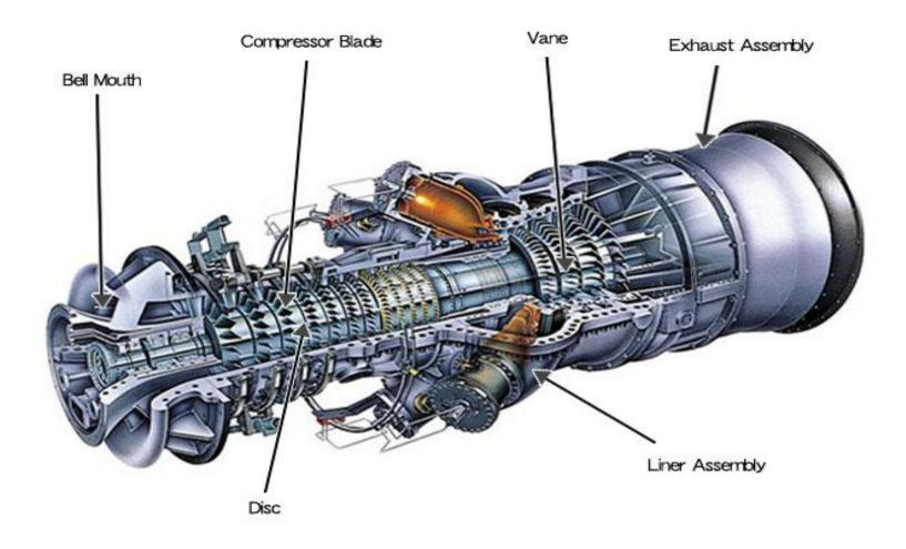
A gas turbine engine is very light and easily removed for maintenance. It is also suitable for complete automation.
