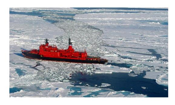
Nuclear power in ship has mainly been confined to ice-breakers. A nuclear-powered ship differs from a conventional turbine ship in that it uses the energy released by the decay of radioactive fuel to generate steam. The steam is used to turn a shaft via a turbine in the conventional way.
