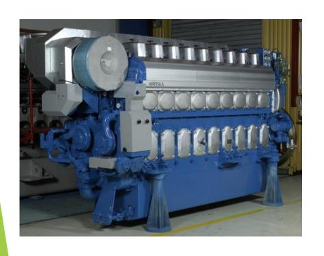
More and more of the larger merchant vessels are being powered by *medium-speed diesel engines*. These operate between 150 and 450 r.p.m, therefore they are connected to the propeller by gearing. They are cheaper than slow-speed diesel engines, and their smaller size and weight can result in the smaller cheaper ships.
