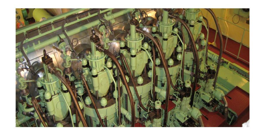
The MAN B&W 5S50MC 5-cylinder, 2-stroke, low-speed marine diesel engine.
