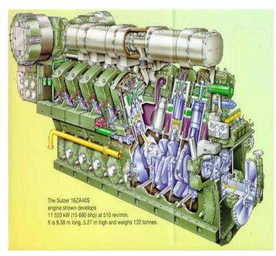
The diesel engine is a form of internal combustion engine.
