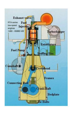
Large diesel engines, which have cylinder nearly 900 mm in diameter, turn at the relatively slow speed of about 145 rpm and less. They are known as low-speed diesel engines. They can be connected differently to the propeller without gearing. Although higher power could be produced by higher revolutions, this would reduce the efficiency of the propeller, because the propeller is more efficient the larger it is and the slower it turns.
