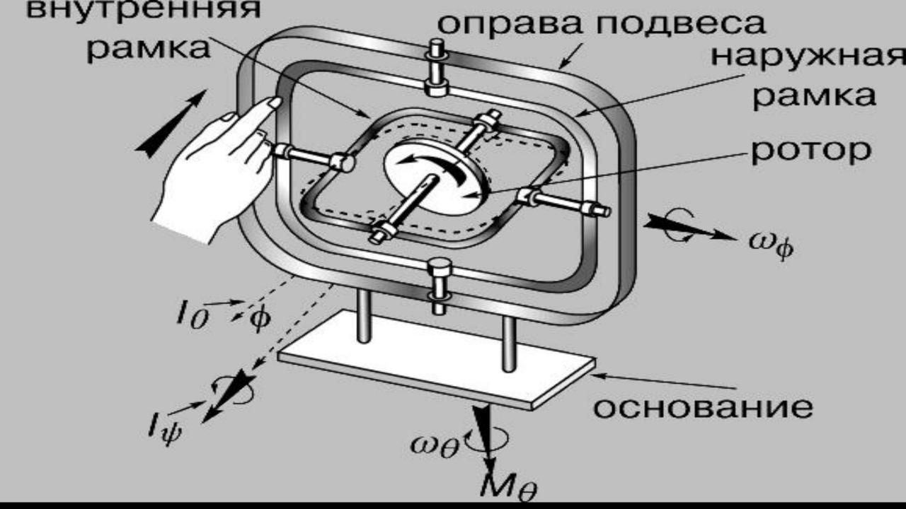
• The two fundamental properties of a gyroscope are rigidity in space and precession. Rigidity is the characteristic that makes a gyroscope point in the same direction with respect to space.
