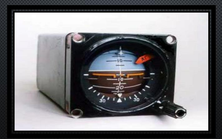
The strip on the dial indicates the inclination of the aircraft forward and backward in the UP or down direction. The pointer on the same dial also shows a lateral tilt in both directions.
